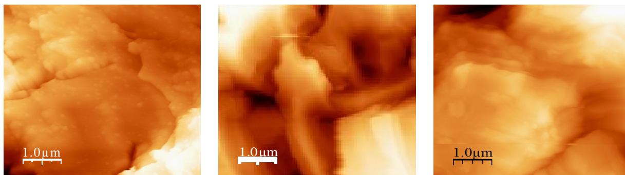
Figure 6. AFM micrograph images of 0.5 thick TiO 2 film on PS. AFM images for bare mc-S and PS/mc-Si are reported for reference.
