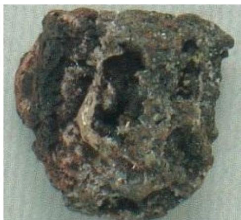
Figure 3. Obtained \text{CuInGaSe}_2 ingot.
